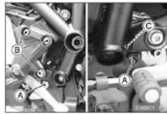
Tighten the bolts while lifting the center stand [A].
