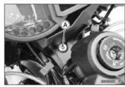
Pull the upper fairing upward to clear the holes [A] from the mirror mounting portions.
