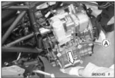
If necessary, prepare a new swingarm mounting plate [A] to hold the engine with the engine stand.
